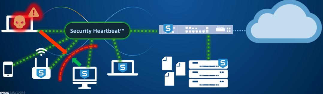
The WIFI Access Point does not allow the infected client to connect to the wireless network
